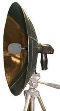
**Figure 10: Parabolic Microphone**
