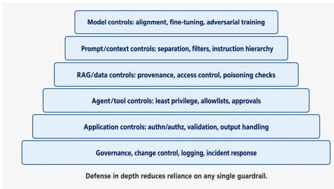
Figure 3. Layered remediation model. Strong AI security places controls around the model as well as inside it.
